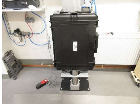
Figure 4: Setup Drop Tests, exemplarily
