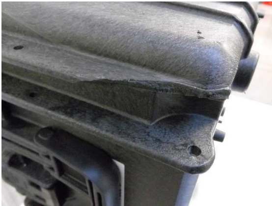
Figure 8: Flaking Bar Corner 3-4-5
