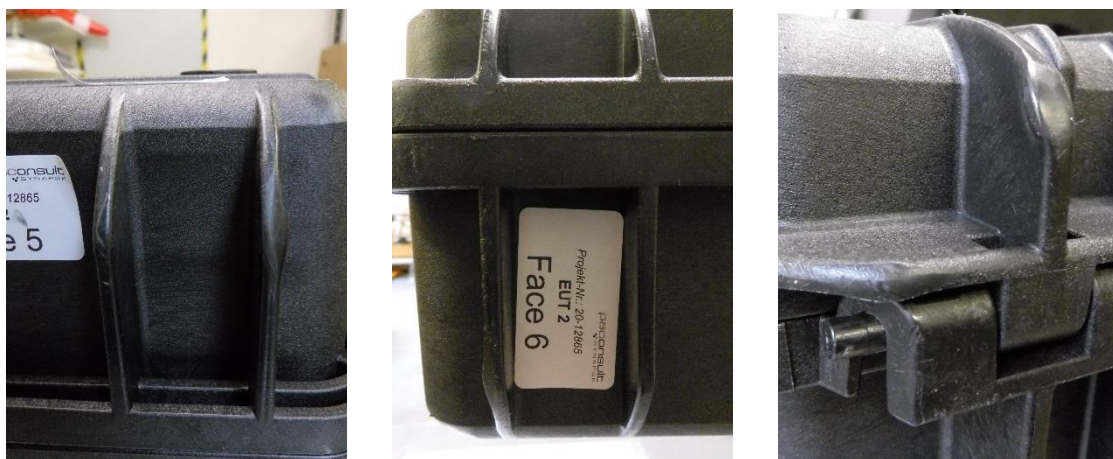
Figure 6: Damaged Bars and Loosened Hinge Pin
